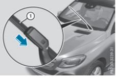
Position new wiper blade 1 in the retainer on the wiper arm and slide it into place in the direction of the arrow. The wiper blade audibly opgages
