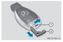
Push release catch (1) in the direction of the arrow and, at the same time, remove emergency key element (2) from the key.
