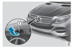
Reach into the gap, pull bonnet catch handle ② up and lift the bonnet. If you lift the bonnet by approximately 40 cm, the bonnet is opened and held open automatically by the gas-filled strut.
