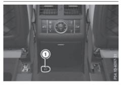
On vehicles with the Rear Seat Entertainment System, there are two sockets in the rear-compartment centre console. ▶ Lift up the cover of socket ①.
