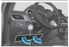
Driver's kneebag (1) deploys under the steering column. The driver's kneebag is triggered together with the front airbags.
