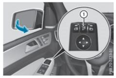
If you have switched on the Auto. fold-in mirrors function and you fold the exterior mirrors in using button (1), they will not fold out automatically ( $\triangleright$  page 118).
