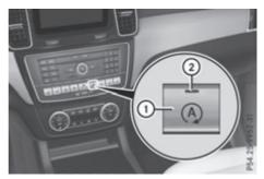
► To switch off: in the Comfort drive program, press ECO button ①.
