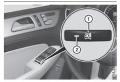
► To activate/deactivate: press button ①. If indicator lamp ② is lit, operation of the rear side windows is disabled. Operation is only possible using the switches in the driver's door. If indicator lamp ③ is off, operation is possible using the switches in the rear compartment.
