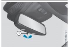
► Anti-dazzle mode: pivot anti-dazzle switch ① forwards or back.
