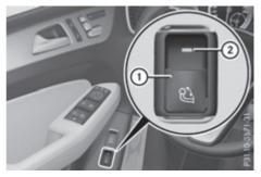
Folding out using the switch in the driver's door (all vehicles except plug-in hybrid vehicles):
