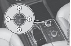
Setting the vehicle level using the selector wheel
