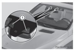
DISTRONIC PLUS with Steering Assist and Stop&Go Pilot aids you in keeping the vehicle in the centre of the driving lane by means of moderate steering interventions in a speed range from 0 - 200 km/h.
