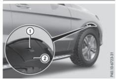
You must remove the cover from the front wheel housing before you can change the front bulbs.
