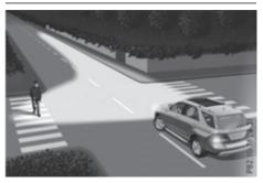
The cornering light function improves the illumination of the road over a wide angle in the direction you are turning, enabling better visibility in tight bends, for example. It can only be activated when the dipped-beam headlamps are switched on.
