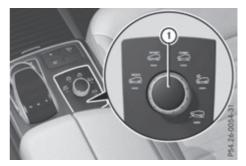
All vehicles (except Mercedes-AMG vehicles): turn DYNAMIC SELECT controller (1) as many times as necessary until the desired drive program is selected.
