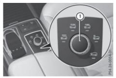
In the **Comfort** drive program, the driving characteristics of your vehicle are more comfortable. Therefore, select this drive program if you prefer a more comfortable driving style. Also select the **Comfort** drive program when driving fast on straight roads, e.g. on straight stretches of motorway.  Select the Comfort drive program using DYNAMIC SELECT controller (1).
