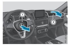
Driver's airbag ① deploys in front of the steering wheel. Front-passenger front airbag ② deploys in front of and above the glove compartment.
