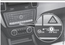
► To prime: lock the vehicle with the key or KEYLESS-GO. Indicator lamp ① flashes. The alarm system is primed after approximately 15 seconds.
