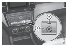
► To switch off: press ECO button ①. Indicator lamp ② and the ④ ECO symbol in the multifunction display go out. ► To switch on: press ECO button ①. Indicator lamp ② lights up. If all conditions for automatic engine switch-off (▷ page 162) are fulfilled, the ③ ECO symbol is shown in green in the multifunction display.
