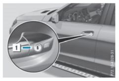
► Turn the emergency key element anti-clockwise to position 1. On right-hand-drive vehicles, turn the emergency key element clockwise. The door is unlocked.
