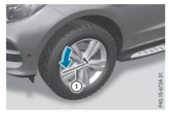
Using wheel wrench ①, loosen the bolts on the wheel you wish to change by about one full turn. Do not unscrew the bolts completely.
