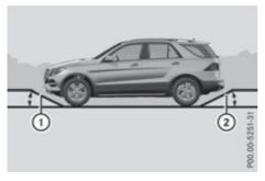
The table shows approach and departure angles (1) and (2) when the vehicle is loaded and ready to drive.
