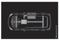
The electric motor is being operated as an alternator, e.g. in overrun mode and when braking. The kinetic energy of the vehicle is converted into electrical energy. The high-voltage battery is charging.
