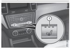
The three blue indicator lamps in the buttons indicate the ventilation level you have selected.
