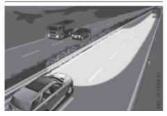
Motorway mode increases the range of the beam.
