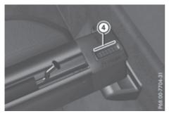
Make sure that the red lock verification indicator ④ is no longer visible. The combined luggage cover and net will otherwise not be locked in place.
