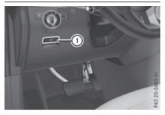
To ensure that you do not roll backwards when pulling away on an uphill slope, apply the electric parking brake. ▶ Press and hold handle ①.
