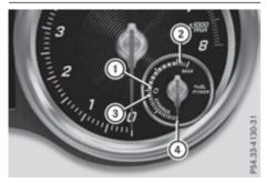
The electric motor power display is on the righthand side of the instrument cluster.
