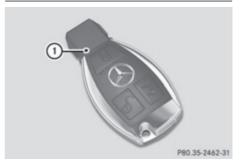
► Press the or button. The battery is OK if battery check lamp () lights up briefly.
