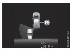
If a course-correcting brake application occurs, red warning lamp (1) flashes in the exterior mirror and a dual warning tone sounds. In addition, display (2) underlining the danger of a side collision appears in the multifunction display. In very rare cases, the system may make an inappropriate brake application. A course-correcting brake application may be interrupted at any time if you steer slightly in the opposite direction or accelerate.
