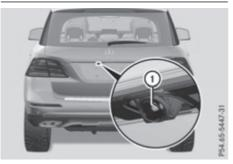
Reversing camera 1 is an optical parking and manoeuvring aid. It shows the area behind your
