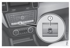
► To deactivate: press button ①. The S<sub>F</sub> ESP<sup>®</sup> OFF warning lamp in the instrument cluster lights up. ► To activate: press button ①. The Stress Defension of the instrument cluster goes out.
