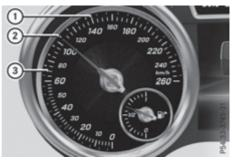
Example: DISTRONIC PLUS displays in the speed-ometer
