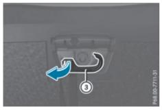
Fold out hook (3) on the underside of the luggage compartment floor in the direction of the arrow.
