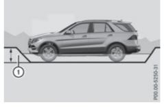
The table shows fording depth ① when the vehicle is loaded and ready to drive.
