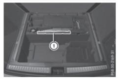
Warning triangle (1) is located in the stowage well under the luggage compartment floor.
