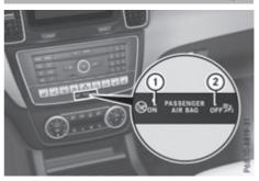
PASSENGER AIR BAG ON indicator lamp (1) and PASSENGER AIR BAG OFF indicator lamp (2) are part of the automatic deactivation system of the front-passenger front airbag.
