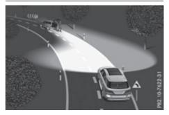
The active light function is a system that moves the headlamps according to the steering movements of the front wheels. In this way, relevant areas remain illuminated while you are driving. This allows you to recognise pedestrians, cyclists and animals.
