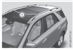
Secure the roof carrier to roof rails (1). In doing so, observe the manufacturer's installation instructions.
